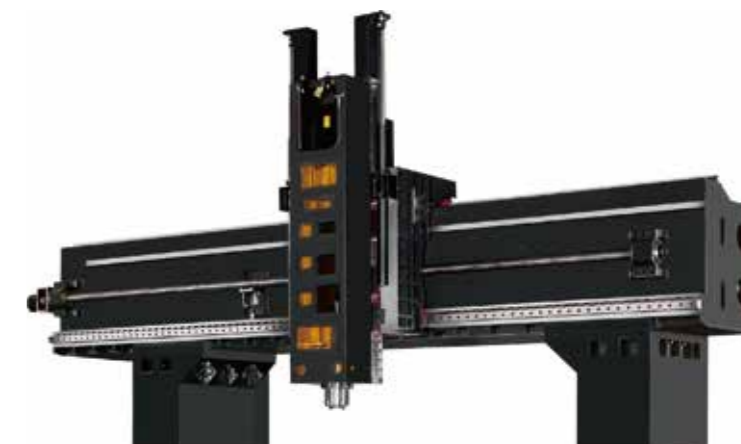
Distance between columns over 3.5m
