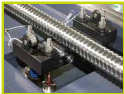
Ball-screw support unit for travel over 5m in X axis.
