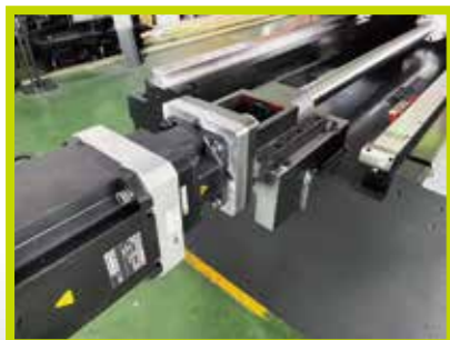
Germany made planetary gearhead represents stability and accuracy.
