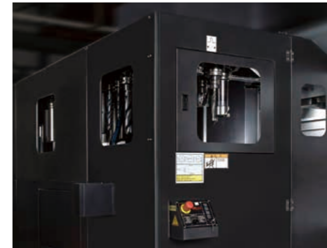
• 32 tools tool magazine (STD); 60,90 tools as option.
