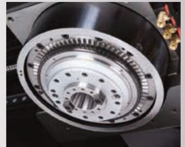
• Index mechanism in every 5 degree for automatic multi-head. (OPT)
