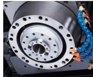
• Index mechanism in every 90 degree for manual multi-head. (OPT)
