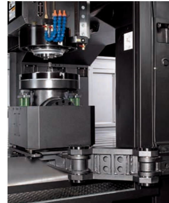
• Swing type one head storage on the right column. (OPT)
