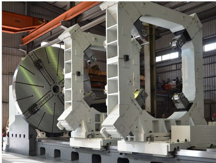
Heavy duty steady rest / Dia. 520mm tailstock
